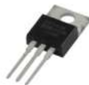
Fig. 7 Mosfet as switch (irf540n)
